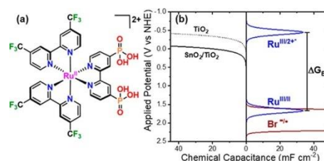
Figure 1. (a) Ru(btmbf) 2 P photocatalyst. (b) Density of states for ground and excited states of surface-bound Ru(btmbf) 2 P photocatalyst (blue), the one-electron Br - redox couple (brown), and the mesoporous thin acceptor states of TiO 2 and SnO 2 /TiO 2 CS (gray).
